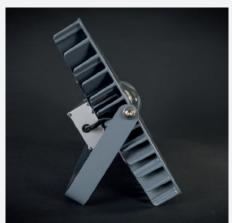
Beam Angle **Light Source** Voltage Efficiency **Luminous Flux Model Number** CCT Power VERSO-65W-5000K 65W COB LED 85-265v AC 125 lm/w 8500lm COB LED 10220lm 85-265v AC 125 lm/w VERSO-90W-5000K 90W 120° or 80° 5000k VERSO-120W-5000K 120W COB LED 85-265v AC 110 lm/w 13213lm VERSO-150W-5000K 150W 85-265v AC 16703lm COB LED 111 lm/w
